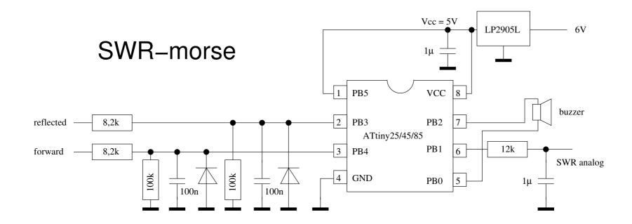
The SWR is output in Morse code and as voltage between 1V an 5V.
